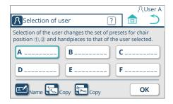
2. On the "Selection of user" screen, press the switch for the user memory for selection and name registration. (In this example, User memory A is selected.)
