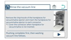
6. Open the front panel of the cuspidor unit. Pick up the vacuum and saliva ejector handpieces from the assistant holder and insert them into the connector.
