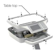
2. Remove the seven screws and detach the table top.
