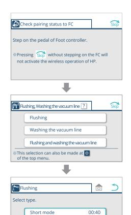
Hold down the pedal of the wireless foot controller until the flushing screen appears.
