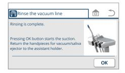
3. After rinsing of the vacuum line is completed, press the ok switch.
