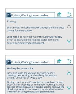
Explanation of flushing and washing the vacuum line
