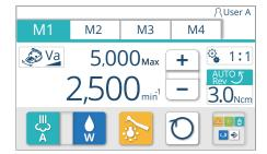
Memory setting for starting condition after powering on (NBX/NLX plus/NLX nano/MX2/MCX)
