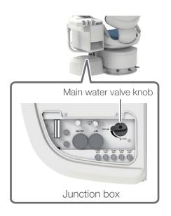
Turn the main water valve knob counterclockwise until the knob is positioned vertically.
