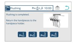
When flushing is completed, rinsing of the vacuum line will start.
