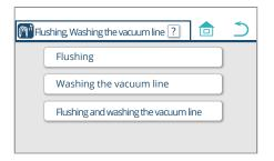
3. Press the 'Flushing' switch.
