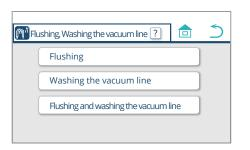
3. Press the 'Flushing' switch.
