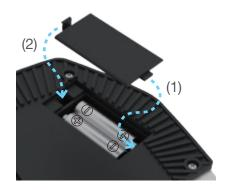
3. Insert two new/charged AA batteries into each box. Use alkali dry batteries or NiMH batteries.
