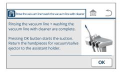
3. When you have finished rinsing the vacuum line+washing the vacuum line with cleaner, press the ok switch.
